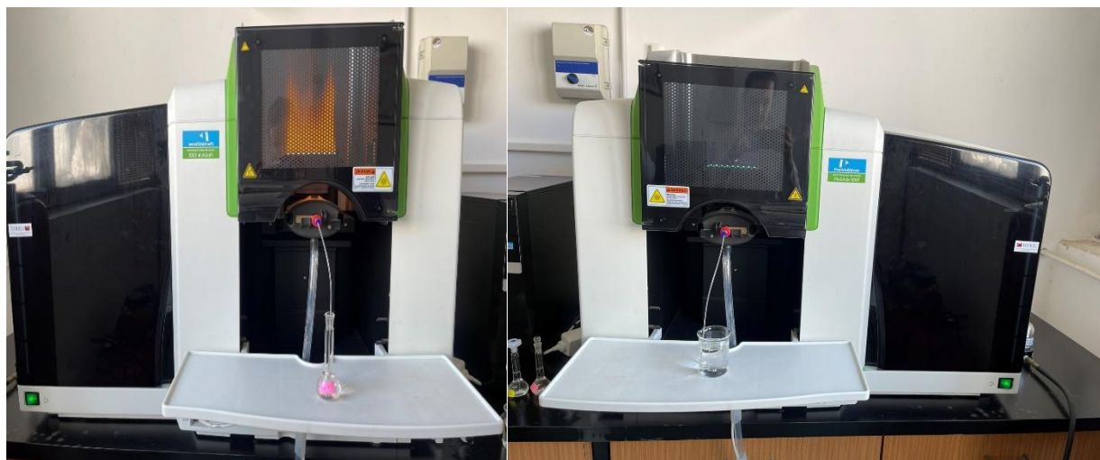
Slika 14. Atomski apsorpcioni spektrometar (AAS -Atomic Absorption Spectrometer- Perkin Elmer PinAAcle 900F).
