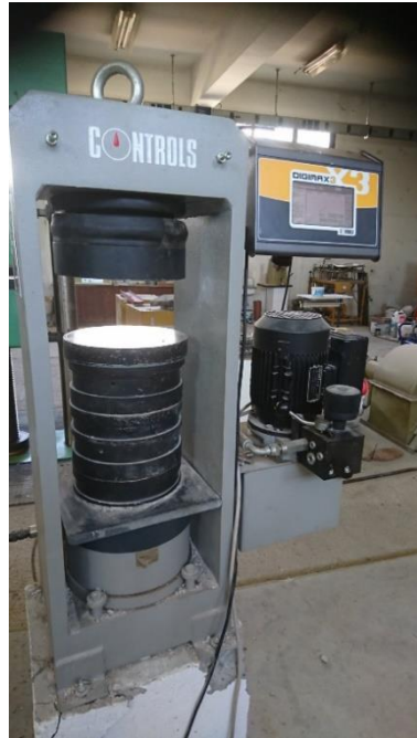
Slika 13. Presa tipa CONTROLS 20063 Cernusco s/N. Milano-Italy
